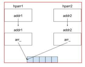
The default copy constructor does a shallow copy of the fields, so hparr2's arr\_ points to the same array as hparr1's arr\_. When hparr1 gets deleted, so does its arr\_. But this arr\_ is the same one hparr2's arr\_ points to, so when hparr2 gets deleted, its arr\_ has already been deleted, leading to an invalid delete (similar to a double free ()).
